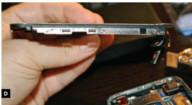
Fig. C: Touchscreen and frame pried away. Fig. D: Touchscreen and 3 cables detached.
