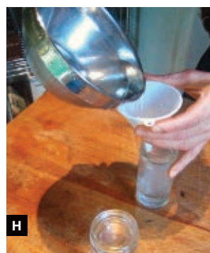
Fig. E: The receiving bowl must be centered and level. Figs. F and G: Place the ice-filled condensing bowl over the receiving bowl. Fig. H: Pour the contents into a different container each time you harvest.
