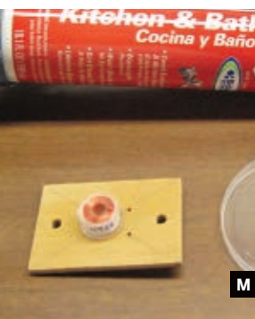
Fig. J: Prepare tape to wrap around bobbin. Fig. K: Use a magnetic compass to find the polarity of each magnet. Fig. L: Pickup mounting board with brass escutcheon pins. Fig. M: Bobbin mounted with a dab of adhesive.
