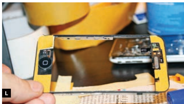
Fig. I: Separating the broken glass from the frame after heating. Fig. J: The frame after removing the glass and the old adhesive, and cleaning it with acetone or electronics cleaner spray.
