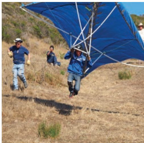
GUMPTION GLIDERS: (Above) A short but successful flight on our PVC and tarp version. (Left) The 1970 photo that inspired our build: Bob and Chris Wills flying Bamboo Butterfly hang gliders designed by Richard Miller.
