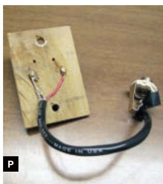
Fig. N: Solder bobbin wires to pins. Fig. O: Prepare a short length of shielded cable by removing a bit of insulation from each end. Fig. P: One end of the cable was soldered to the pins and the other to the lugs of the phono jack.
