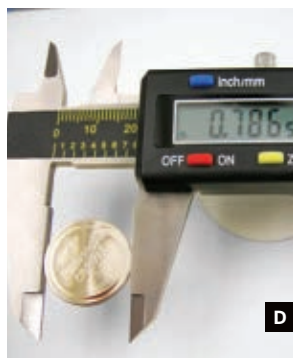
Fig. A: Calipers give an accurate inner diameter of your yo-yo. Fig. B: Set the compass cutter to match the inner radius. Fig. C: Cut the side cap out of sheet plastic. Fig. D: Measure your coin cell battery, then lightly scribe
