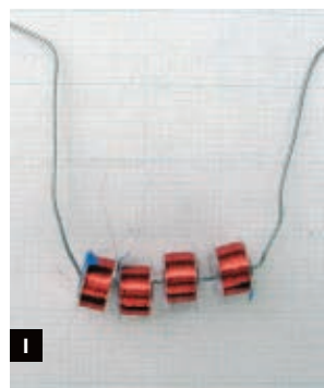
in the top of the bobbin. Fig. D: The weight provides friction resistance. Fig. E: Bobbin filled with wire. Fig. F: Tape wire to the top of the bobbin. Figs. G and H: Melt wax in hot water — outside. Fig. I: Bobbins ready to dip in wax.
