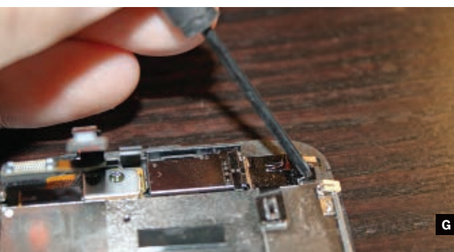
Figs. E, F, G: Unscrew 5 tiny screws on the sides and top of the frame to separate the LCD touchscreen from its frame. Some of these screws are hidden under pieces of tape.
