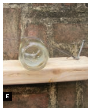
nail, and mark where it rests on the board. Fig. D: Rasp out a groove for the jar to fit into. Fig. E: Slip the jar back so it snaps into the groove. Fig. F: Use a hammer with a dowel to whack the wooden nut into place.
