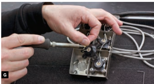
Fig. F: Electret condenser microphone. The ground lug connects to the casing; the signal lug doesn't. Fig. G: Soldering the electret condenser microphone.
