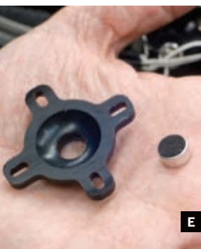
Fig. C: Headgear cells. Fig. D: Mic cell, showing cartridge and spring mechanism. Fig. E: Electret condenser microphone and custom-designed cartridge.
