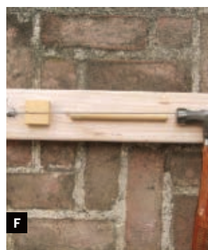
nail, and mark where it rests on the board. Fig. D: Rasp out a groove for the jar to fit into. Fig. E: Slip the jar back so it snaps into the groove. Fig. F: Use a hammer with a dowel to whack the wooden nut into place.
