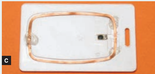
Fig. A: Removing part of the shell reveals the tiny circuit board and damaged coil. Fig. B: The old, donor card. Its coil is intact, but its chip contains the wrong code. Fig. C: The good chip soldered to the donor coil, in its case.
