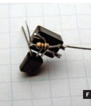
Fig. D: Solar battery with the Schottky diode and supercap soldered in. Fig. E: Solder the transistor collector (C) and base (B) to pins 2 and 4 of the transformer. Fig. F: Solder the resistor between pins
