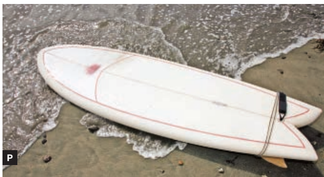
edge in the tail. Fig. O: Drip resin around the leash plug, wait awhile for bubbles to rise, then drip a little more if needed. Fig. P: Your board will be strongest if you let the epoxy cure 7 full days — if you can wait that long.
