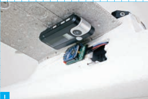
ANATOMY OF AN UNMANNED AERIAL VEHICLE: Fig. C: The assembled DIY Drone. The parts to build one cost about $300. Fig. D: The ArduPilot autopilot system is based on the Arduino open source hardware platform. Fig. E: The GPS module used for navigation. Fig. F: XY sensor for stabilization. Fig. G: Z sensor for stabilization. Fig. H: Z sensor and servo mounted on UAV. Fig. I: Digital camera and XBee wireless module (for real-time wireless telemetry). Fig. J: Close-up of XBee telemetry system.
