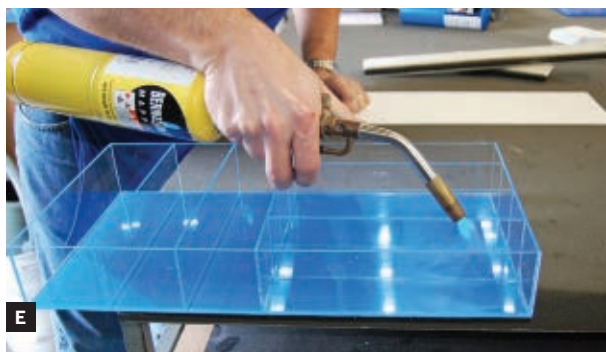
scraps to maintain right angles. Fig. D: Weights help maintain good contact while the glue sets. Fig. E: For the finishing touch, break out the gas torch for a professional-looking flame polish!
