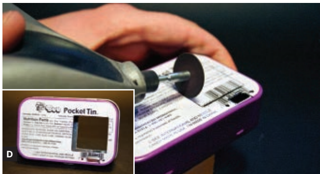
soldering, to insulate all connections from the conductive metal tin. Fig. C: It's a snug fit. Fig. D: Use light pressure when cutting the openings; let the tool do the work. The openings don't have to be perfectly aligned.
