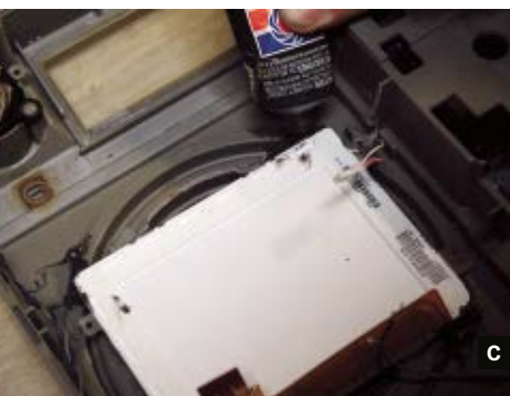
Fig. A: The Sony PSone screen is a great, hackable display perfect for installing in a boombox. Fig. B: Use a Dremel tool to cut out a rectangle in the speaker grill to accommodate the display. Fig. C: Use RTV black
