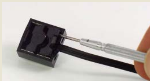
Fig. A: Pry off the back panel of the Lego 9V motor wire bricks using a small screwdriver. Discard or save the wire, as you won't need it for this project.
