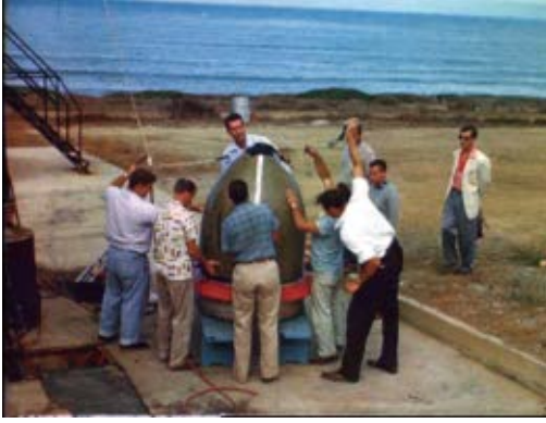
ABOVE: Tethered testing of a 300-lb 1-meter-diameter high-explosive driven flying model at the Point Loma test site, summer 1959. Present that day were Freeman Dyson (carrying briefcase) along with (clockwise from top) Ed Day, Walt England, Brian Dunne, Perry Ritter, Jim Morris, Michael Feeney, W.B. McKinney, Michael Ames. SEQUENCE AT RIGHT: Free flight testing, October 1959. The initial kick is given by a 1-lb charge of black powder; the subsequent 5 charges each contain 2.3 lbs of C-4.
