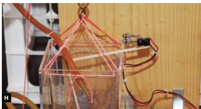
thinner air (increases with altitude). Figs. G & H: To simulate stalling, a low float level in Kinetic pulls a lever that opens a solenoid valve and switches on a warning light ( Figs. I & J. )
