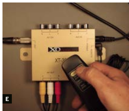
silicone from the auto parts store as a glue to attach the display to the boombox. Fig. D: Heed all warning signs regarding electricity! Fig. E: An RF tuner provides a television signal.
