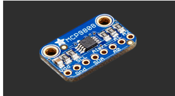
Figure 27-12 The Microchip MCP9808 on a breakout board from Adafruit.
