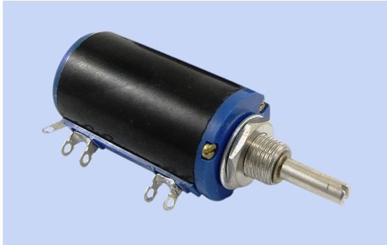
Figure 7-2 A multiturn rotary potentiometer. Each pair of solder tags is attached internally to one end of the internal coiled track. The smaller tag at the far end connects with the wiper.
