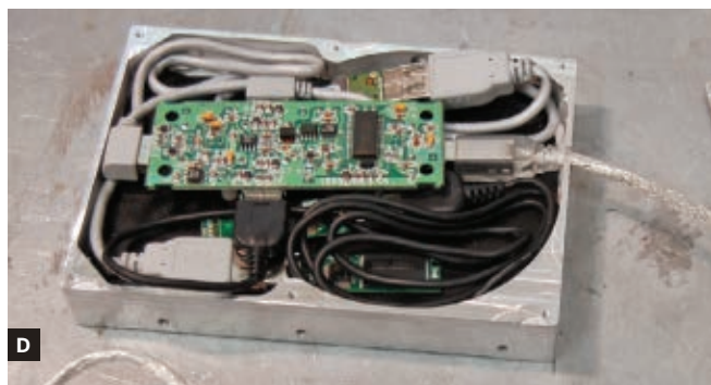
Fig. C: Pry apart the USB hub case and remove its board. Fig. D: Memory sticks, cables, and USB hub packed into the hard drive case. The external USB cable exits a hole drilled in one end.
