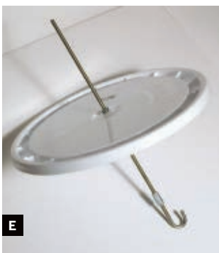
connect all 4 anodes with a wire. Fig. D: Use zip ties to connect the anodes to the mesh. Fig. E: Drill a hole in the center of the lid and insert the threaded rod. Fig. F: Drill lots of ventilation holes for gases to escape.
