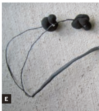
stereo plug in opposite directions, with ground (in back) connecting to blue on one, red on the other. Plug tip is the right channel, and sleeve (middle) is left. Fig. E: The finished microphone passes as earbuds.
