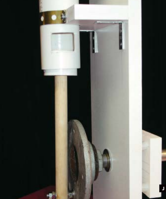
Fig. J: Cylinder and moving parts installed: piston, rod, crank, crankshaft, and flywheel (not shown).
