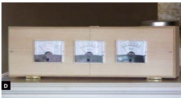
Fig. C: Holes in the box, with some holes sawed out into slots to fit screws. Fig. D: The meters with their new scales fit into the box.
