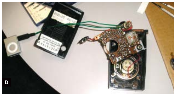
Fig. C: Convert stereo to mono by adding resistance to channels and connecting them together. Fig. D: The iPod connected and the radio ready for reassembly.
