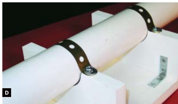
Fig. C: Cylinder saddles mounted to front bearing block and lined with adhesive tread. Fig. D: Cylinder test-mounted in saddles with brass pipe strapping hold-downs.
