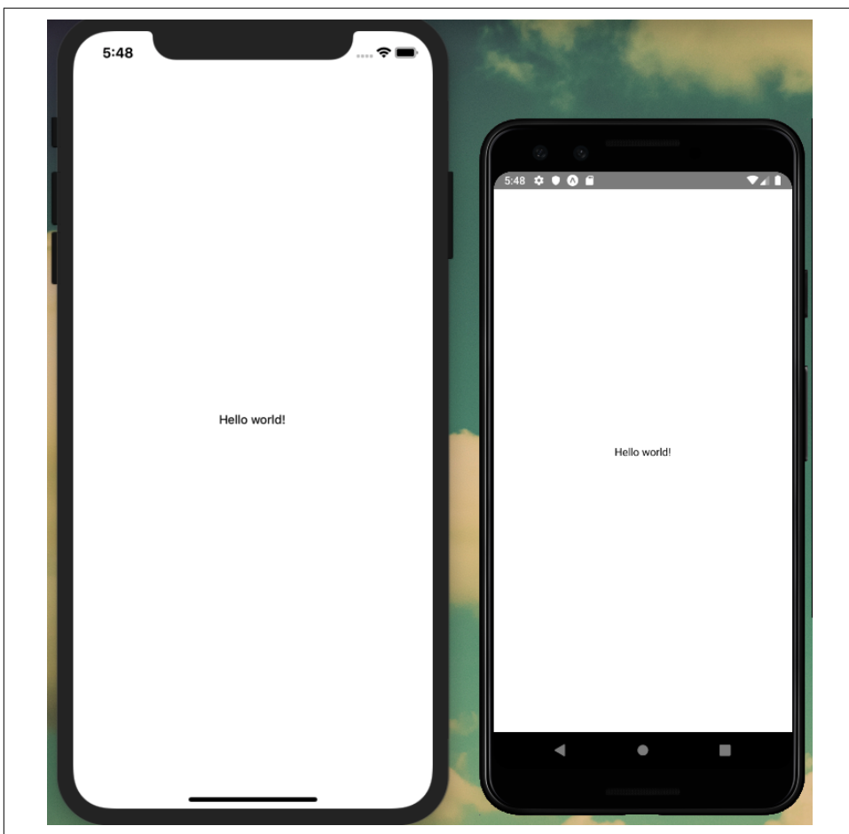
Figure 21-2. Our application running side by side on iOS and Android device simulators
