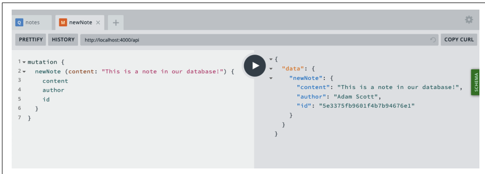
Figure 5-2. A mutation creates a new note in the database
