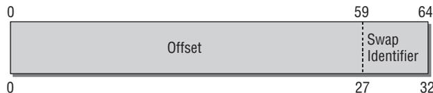
**Figure 18-6: Components of an architecture-independent swap identifier.**
