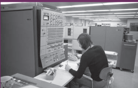
The original 360 was the IBM System/360, a highly successful mainframe computer “family” produced from 1965 to 1978. Shown here is a unit installed for the Volkswagen automobile company. Source: German Federal Archive.
