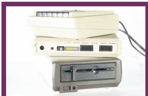
From top to bottom, the Atari 410 Program Recorder (tape drive), the Atari 850 Interface module (showing two SIO ports), and the Atari 1050 disk drive.
