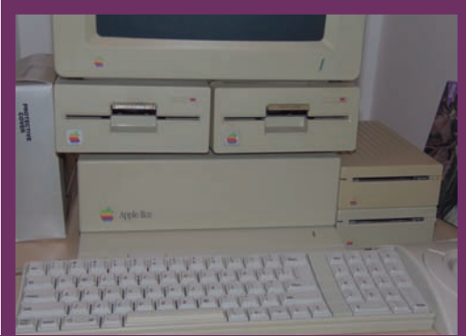
An Apple IIGS with a full complement of disk drives and third party trackball. The IIGS was the first Apple II series computer with a detachable keyboard.
