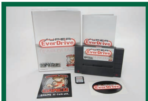
A deluxe version of the Krikzz Super Everdrive from reseller Stone Age Gamer. Most NTSC and PAL games are directly supported, save for those requiring special chips.
