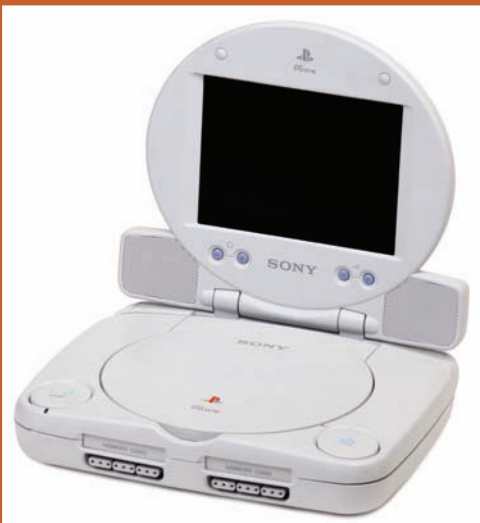
The compact PSone with its optional 5-inch diagonal LCD screen attachment. The actual console is approximately the same width as the standard controller. Courtesy of Evan-Amos, Vanamo Media.
