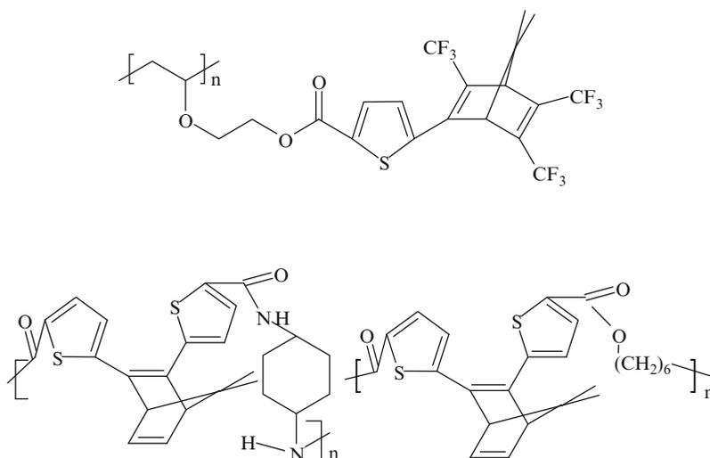
All of the above polymers exhibit large absorption bands in the visible region of the spectra and the norbornadiene moieties in these polymers isomerize very rapidly. In addition, the norbornadiene moieties also exhibit efficient fatigue resistance [185].
