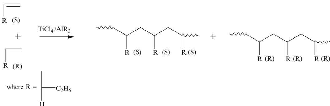
**Fig. 4.4** Two enantiomorphs form of the catalyst. R indicates the ligands that was replaced by alkyl groups through alkylation by organometallic compounds from Groups I through III
