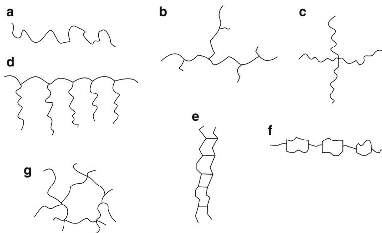
**Fig. 1.1** Shapes of polymer molecules. (a) Linear polymer, (b) branched polymer, (c) star-shaped polymer, (d) comb shaped polymer, (e) ladder polymer, (f) semiladder polymer, and (g) network structure
