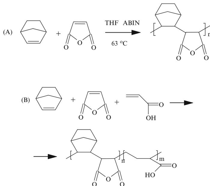
To render the polymers soluble in aqueous base, acrylic acid terpolymerization was also carried out as shown in (B) above.
