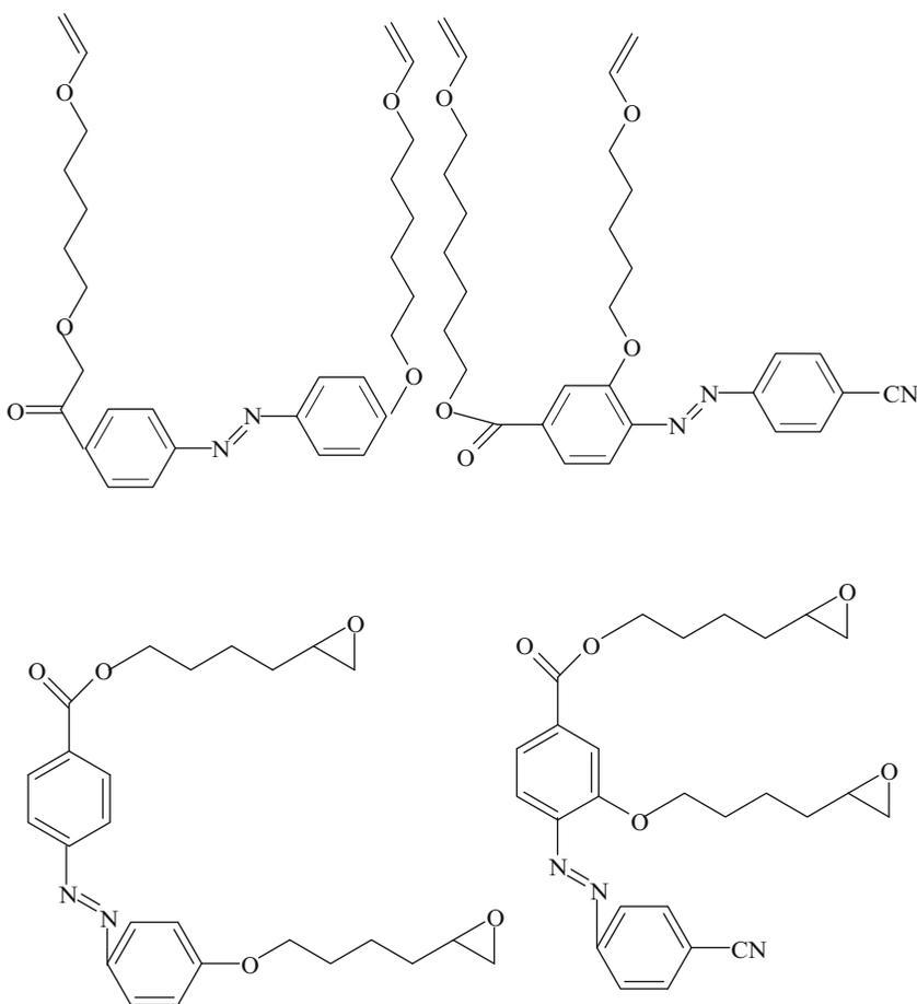
Polymerization of these monomers was achieved by cationic mechanism. The monomers were also found capable of inducing and stabilizing bulk alignment of the liquid crystals. Zhao and coworkers [234–237] concluded, however, that the mechanism of action might be different from the one obtained
