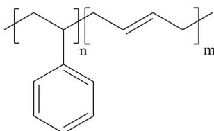
**Fig. 6.4** Illustration of polystyrene and polybutadiene domains
