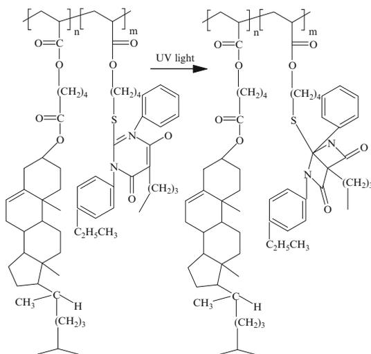
It was found that the rate of photo-rearrangement is affected by the length of the alkyl side group in the 5 position of the pyrimidinium oleate and by the embedding of a chromophore, as shown above [190].
