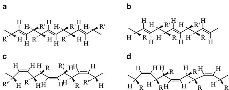
**Fig. 1.3** Tritactic polymers. (a) *Trans-erythro* tritactic polymer, (b) *trans-threo* tritactic polymer, (c) *cis-erythro* tritactic polymer, and (d) *cis-threo* tritactic polymer
