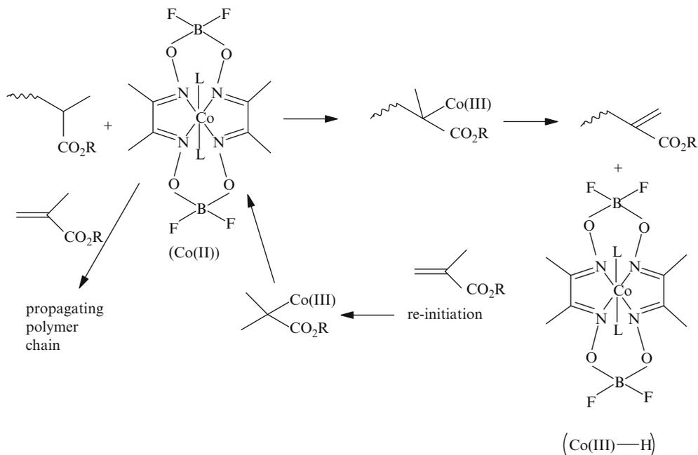
Fig. 3.2 Cobalt mediated controlled/“living” polymerization
