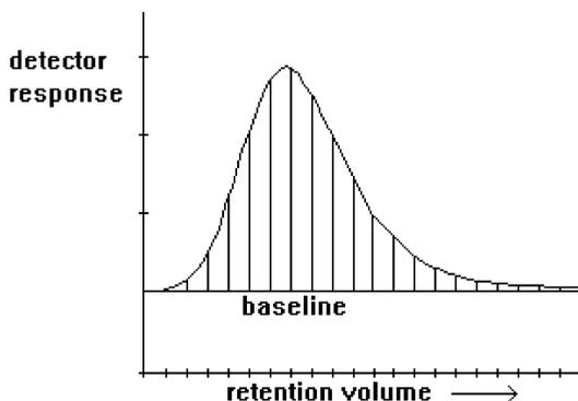
Fig. 2.23 A typical digitized gel permeation chromatogram
