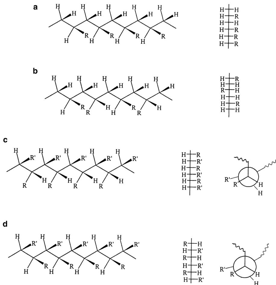
**Fig. 1.2** Steric arrangement in macromolecules ( $R = \text{phenyl}$ ). (a) Isotactic polymer, (b) syndiotactic polymer (c) erythrodiisotactic polymer, and (d) threodiisotactic polymer
