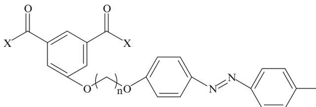
where Y is a hydrogen or a lower alkyl group;  $m = 1-3$ ;  $n = 2-18$ . Polyesters based on this monomers are claimed to be useful for optical recording media such as holograms recording with low light absorption or without loss and wide range of working wavelengths.
