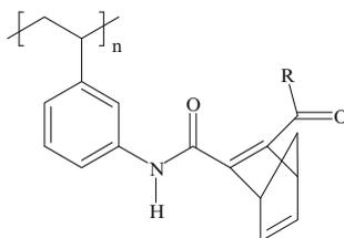
where R is a methoxy or a ring-substituted aniline group attached through the nitrogen or at another position. These pendant groups also undergo reversible conversions into quadricycline units in polymer films when irradiated by ultraviolet light of two different wavelengths. The materials exhibit high photosensitivity as well as a large red-shift in the absorption spectrum upon irradiation.
