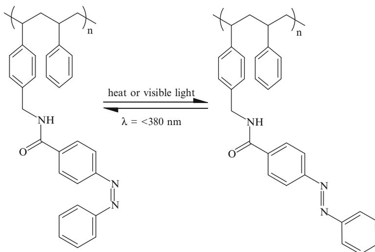
After 10 min of irradiation with ultraviolet light, the photo-stationary state is reached, consisting of 79% of the *cis* isomer. Back isomerization to *trans* of the sample is slow in the dark (less than 10% in 60 min), but is much faster when exposed to visible light [210].
