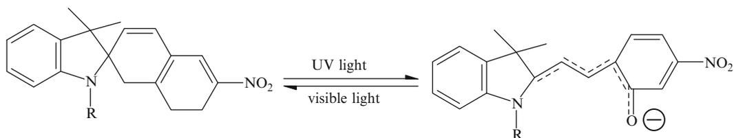
When the irradiation is interrupted and the membrane is irradiated with visible light, the potential returns to its original value, because the ring closes back to the spiran structure [125].
