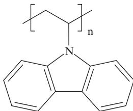
The optical transparency of poly(vinyl carbazole) films produced by this room temperature process appears to be quite high, although transparency decreases at high conversions. In film form, this material is useful for photoconductors, charge-transfer complexes, and electroluminescent devices. The higher polymer molecular weight typically enhances film mechanical properties [247].
