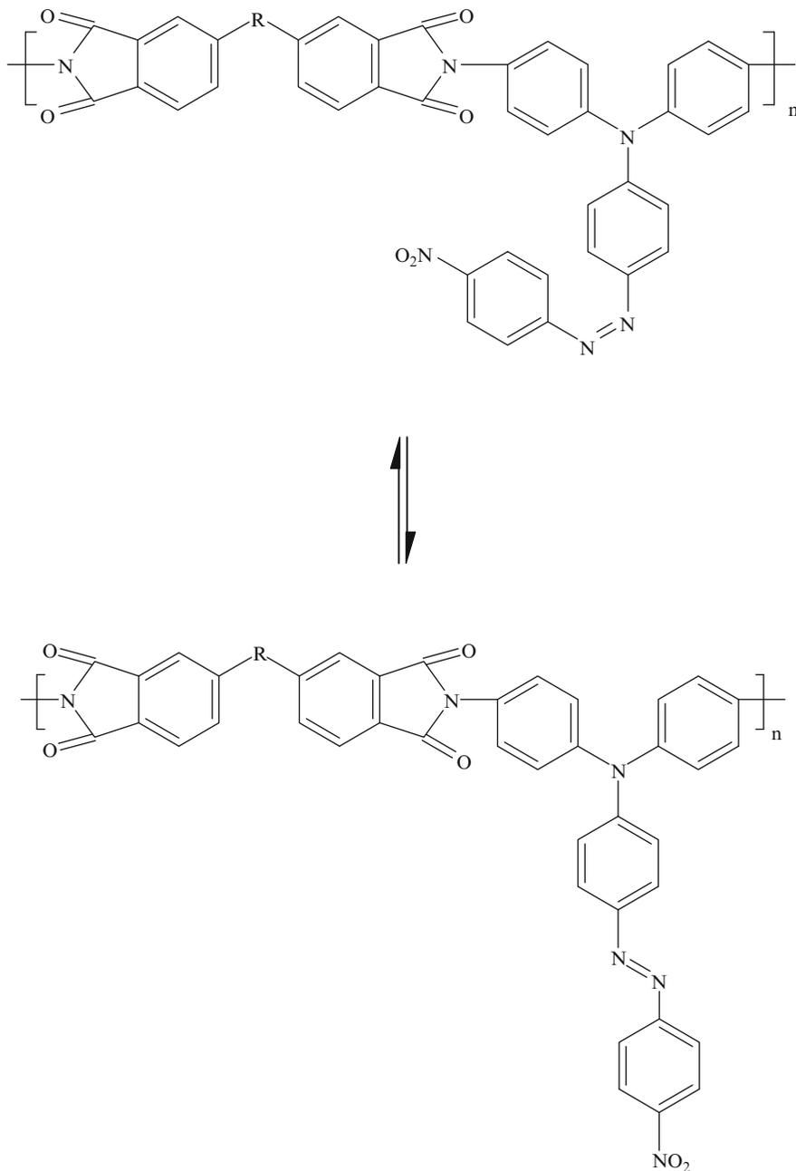
where  $R = (\text{CF}_3)_2\text{C}-$  in one polymer and  $-\text{COO}-(\text{CH}_2)_2-\text{COO}-$  in another.
