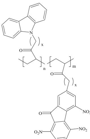
can be prepared by free-radical copolymerization of the appropriate monomers. Photo-conductivity in the visible is obtained by charge transfer complexation.
