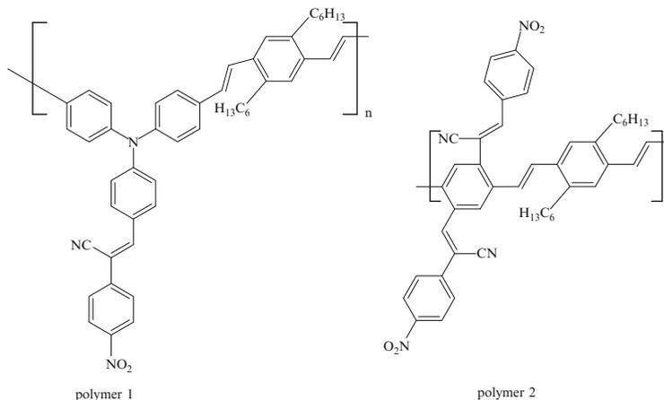
They reported that these copolymers showed broad absorption curves with long-wavelength absorption maximum around 620 nm and optical band of 1.68 and 1.64 eV for both polymers. Both polymers were studied for photovoltaic response in bulk heterojunction solar cells. They observed an overall power conversion efficiency of 3.15 and 2.60% for the cast polymers. Further improvement led up to 4.06 and 3.35% for the devices based on thermally annealed materials.
