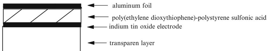
The donor material, containing a chromophore, absorbs the light energy and generates excitons. Excitons are high-energy couples where the energetic electrons are bound to positively charged
