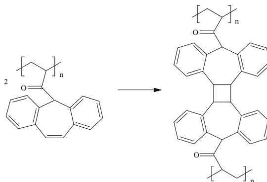
The cross-linking can result from either direct absorption of the light or in the presence of triple sensitizers like Michler's ketone [168]. The  $2\pi + 2\pi$  addition leads to a formation of a cyclobutane cross-link.
