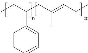
polystyrene block-polyisoprene block
