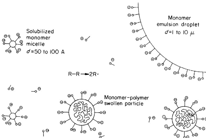
Fig. 3.3 Early stages of emulsion polymerization (from ref. [306])
