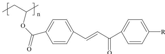
The photosensitivity of this polymer is in the range of 1–5 mJ/cm<sup>2</sup>, according to Watanabe et al. [155]. When the R group shown above is *p*-Br, *m*-NO<sub>2</sub>, or (CH<sub>3</sub>)<sub>2</sub>N, the cross-linking is via formation of biradicals derived from the double bonds of the cinnamoyl groups and an abstraction of protons from the neighboring methyne or methylene groups. This reaction of dimerization can be illustrated as follows [156]:
