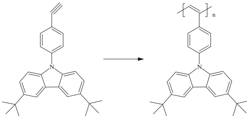
It was found [122] that the current conducted by this polymer during irradiation is 40–50 times higher than it is in the dark. On the other hand, the electron mobility of the di-*t*-butylcarbazolepolyacetylene (shown above) is lower than in poly(vinyl carbazole). This was attributed to the bulkiness of the butyl groups [254].
