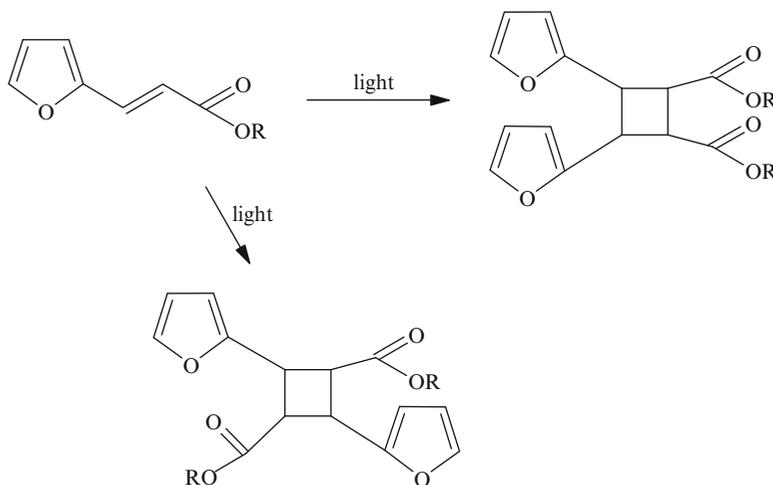
Tajima, Arai, and Takeuchi [161–163] studied the effects of singlet oxygen on photocross-linking of poly(furfuryl methacrylate). The singlet oxygen was generated by fullerene  $C_{60}$ . The reactions were carried out in 1,1,2,2-tetra-chloroethane solutions that contained the polymer and fullerene  $C_{60}$ . Gelation occurs when exposed to visible light in the presence of photosensitizers. These solutions gel after several hours and subsequently solidify completely [163].
