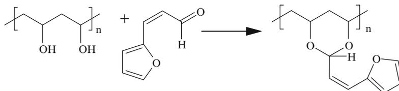
In the presence of photosensitizers, this polymer was found by Tsuda to cross-link at a considerably faster rate than does poly(vinyl cinnamate) [160]. He showed that the cross-linking reaction also results in formation of cyclobutane derivatives. The cross-linking is illustrated on 3-furfurylacrylic ester:
