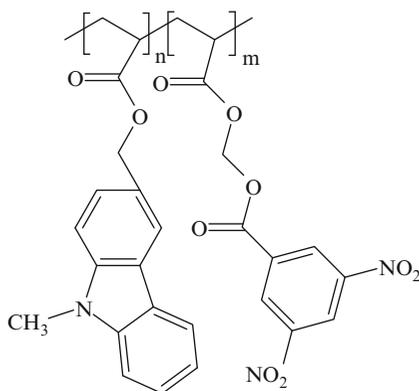
Illumination of the copolymer samples induces a certain degree of ionization accompanied by proton transfer. There is a permanent increase in the quantity of radicals generated by light. Another number of radicals apparently forms during illumination, but disappears in the dark [254].
