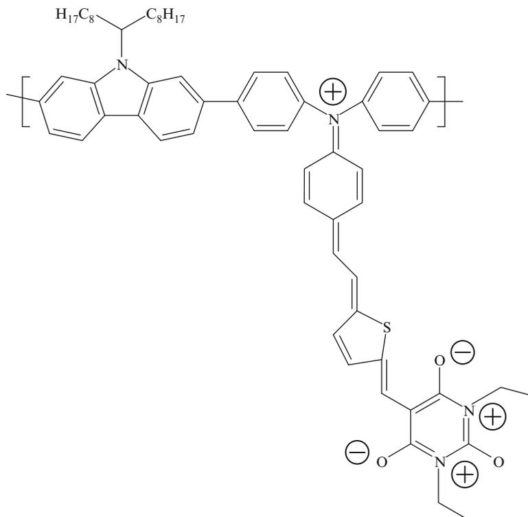
The four copolymers that were synthesized contained different acceptor end groups, aldehyde, monocyano, dicyano, and 1,3-diethyl-2-thiobarbituric acid. Through changing the acceptor groups, the electronic properties and energy levels of the copolymers were effectively tuned. Their results indicate that it is an effective approach to tuning the bandgaps in conjugated polymers. The polymers were used as donors in polymer solar cells. They reported, however, conversion efficiency of only 2.76%.
