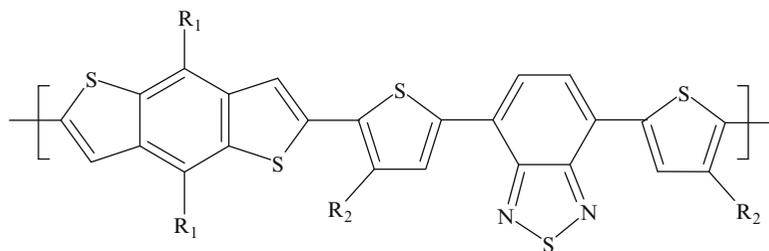
where  $R_1 = 3$ -butylonyl and  $R_2 =$  nonyl and in the second polymer,  $R_1 = 3$ -hexylundecyl and  $R_2 =$  hydrogen.
