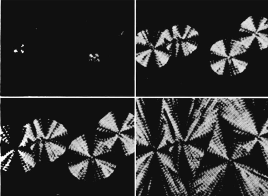
**Fig. 2.13** Spherulitic growth (from ref [50])
