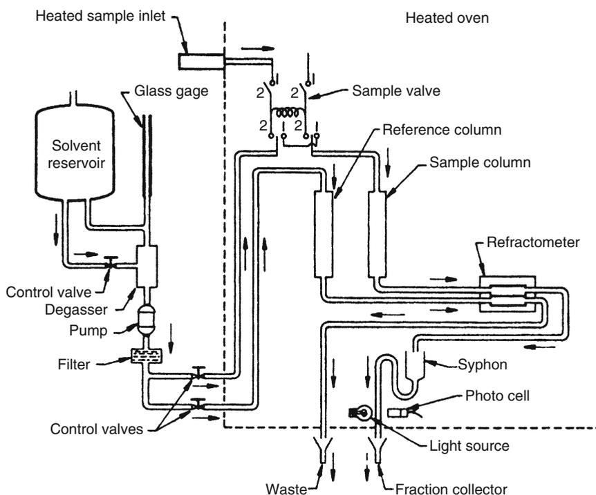
Fig. 2.24 Schematic illustration of gel permeation equipment (the illustration only shows one sample column. Several sample columns are often used) (from ref [68])
