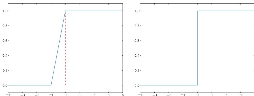
**Fig. 5.8** Plot of the Heaviside function using 9 equally spaced  $x$  points (*left*) and with a double point at  $x = 0$  (*right*)
