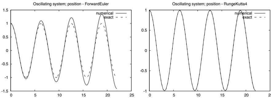
**Fig. E.7** Solution of an oscillating system ( $u'' + u = 0$  formulated as system of two ODEs) by the Forward Euler method with  $\Delta t = 2\pi/200$  (left), and the 4-th order Runge-Kutta method with the same time step (right)
