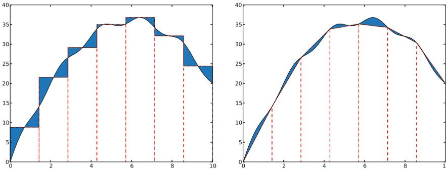
**Fig. 5.22** Visualization of numerical integration rules, with the Midpoint rule to the left and the Trapezoidal rule to the right. The filled areas illustrate the deviations in the approximation of the area under the curve
