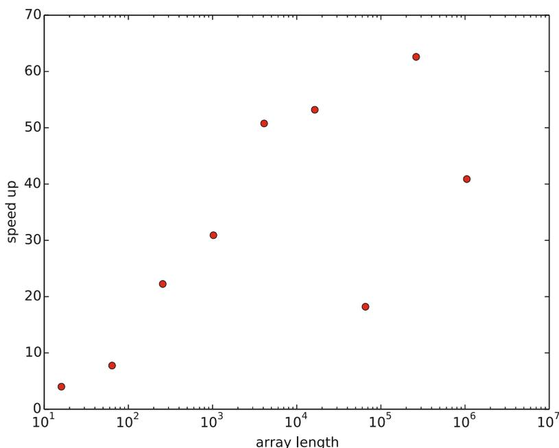
**Fig. 5.11** Improved efficiency of vectorizing the “axpy” operation as function of array length
