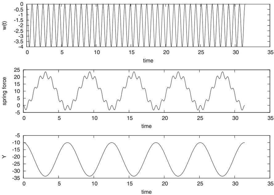
**Fig. D.4** Plot of the plate position  $w(t)$ , the spring force (proportional to  $S(t)$ ), and the position  $Y(t)$  for a test problem where  $w(t) = 2(\cos(8t) - 1)$ ,  $\beta = g = 0$ ,  $m = k = 1$ ,  $S_0 = 0$ ,  $\Delta t = 0.05236$ , and  $N = 600$
