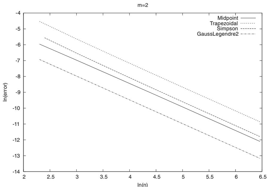
**Fig. 9.5** The logarithm of the error versus the logarithm of integration points for integral  $\frac{3}{2}\sqrt{x}$  computed by the Trapezoidal method and Simpson's rule (*upper two lines*), and Midpoint and Gauss-Legendre methods (*lower two lines*)
