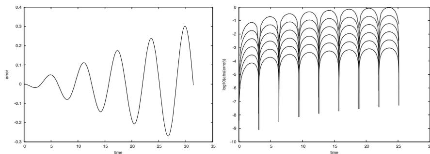
**Fig. D.5** Error plots for a test problem involving an oscillating system: *Left*: the error as a function of time. *Right*: the logarithm of the absolute value of the error as a function of time, where  $\Delta t$  is reduced by one half from one curve to the next one below
