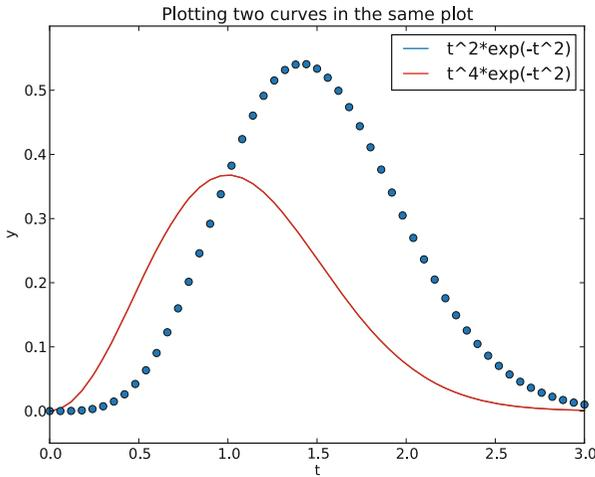
**Fig. 5.4** Two curves in the same plot (Matplotlib)
