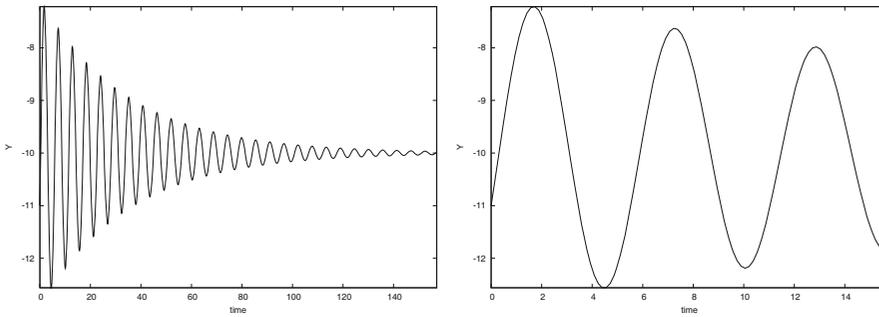
**Fig. D.3** Plot of the position of an oscillating box where the end point of the spring ( $w(t)$ ) is given a sudden movement at  $t = 0$ . Other parameters are  $m = k = 1$ ,  $\beta = 0.1$ ,  $g = 0$ ,  $S_0 = 0$ . *Left*: 1000 time steps. *Right*: 100 steps for magnifying the first oscillation cycles
