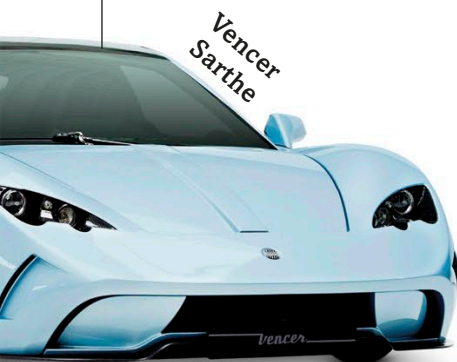
This experimental sports car is built with a rust-resistant alloy that contains molybdenum.
