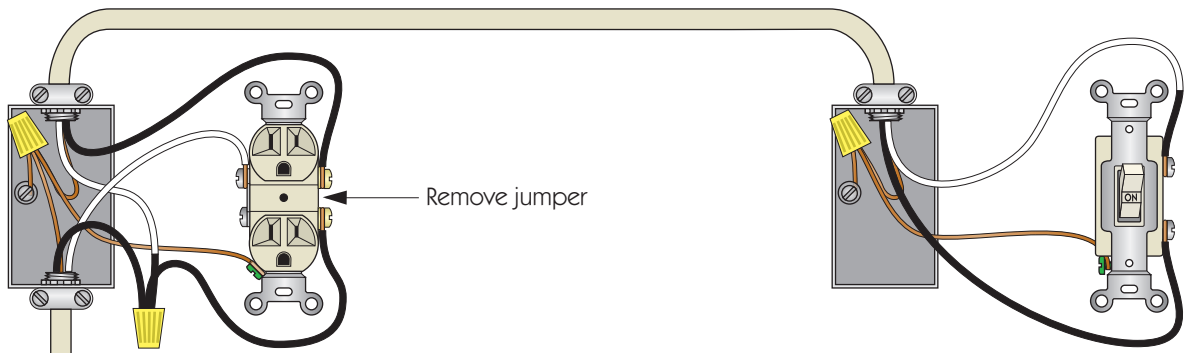
SPLIT-SWITCHED RECEPTACLE (top receptacle switched)
