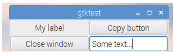
▲ A GtkEntry added to the bottom right of the table
