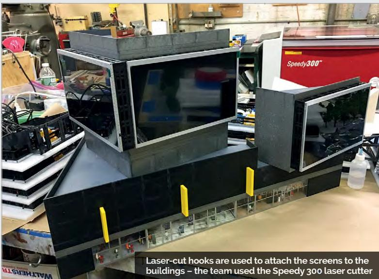
Laser-cut hooks are used to attach the screens to the buildings – the team used the Speedy 300 laser cutter
