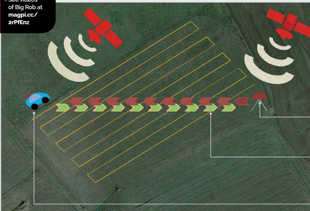
The base station sends its own position to the robot to eliminate GPS inaccuracies caused by atmospheric effects
