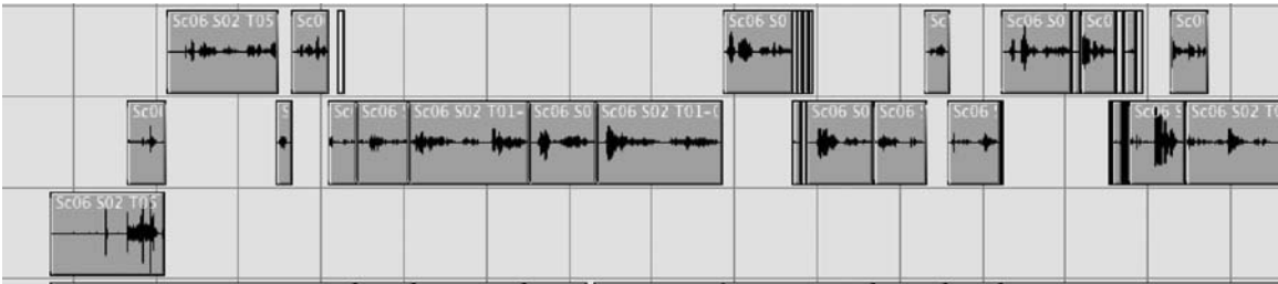
FIGURE 17.7 Tracks split by mic, with the quiet portions deleted.
