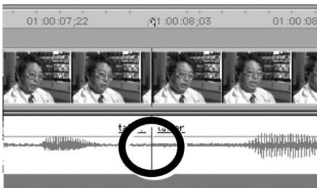
FIGURE 8.3 You can hear room tone jump at this edit point.
