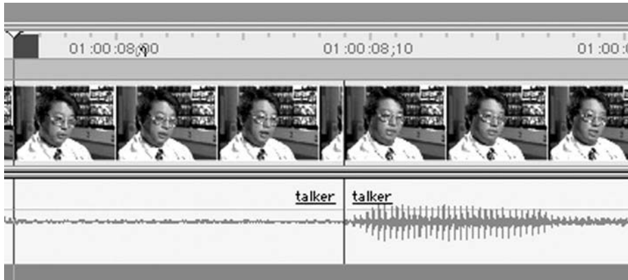
FIGURE 8.4 Rolling the edit to the start of the next sound fixes the problem.
