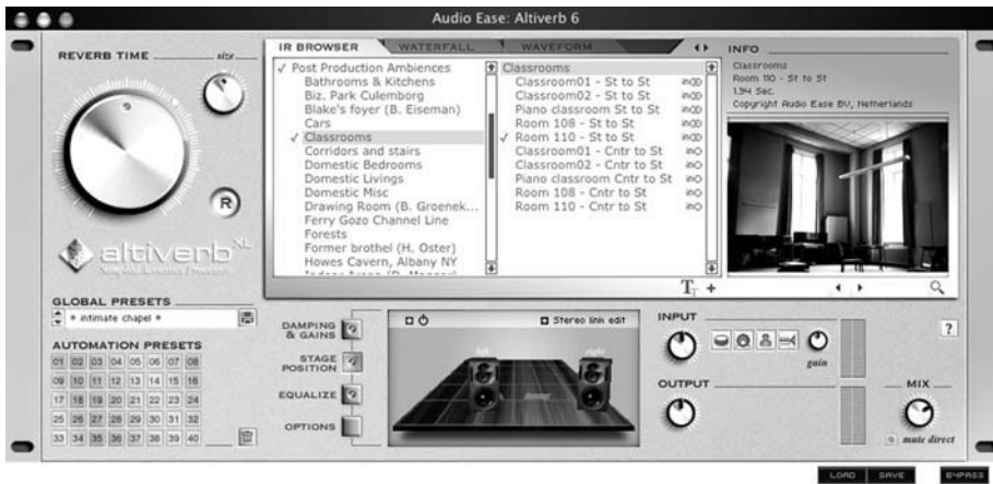
FIGURE 13.10 Altiverb uses recordings of actual reverb in selected spaces, duplicating it on your track.
