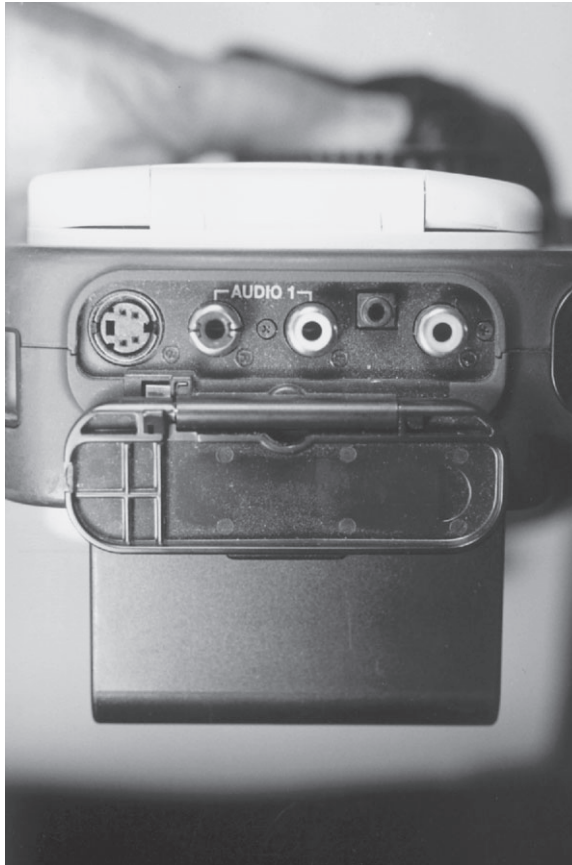
Figure 7-4a An RCA connector pair typically used for consumer analog audio (left channel white, right channel red).
