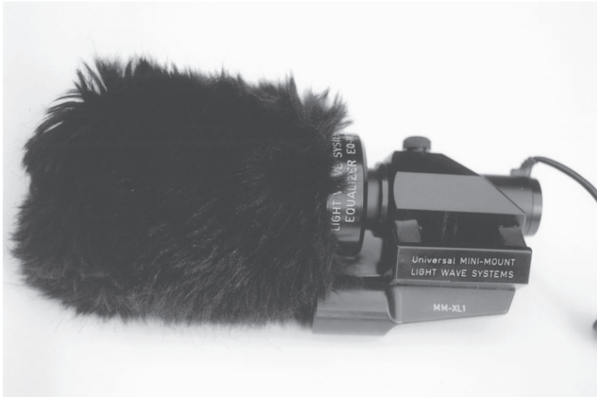
Figure 4-3b Aftermarket windscreen and added shock mount for the Canon XL series cameras offer greater reduction of camera and wind noise than the stock solution.
