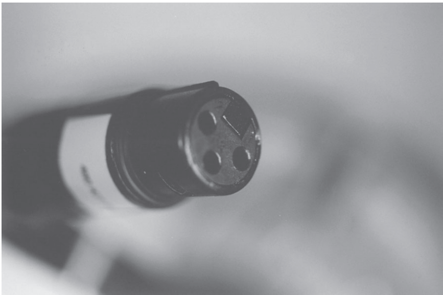
Figure 7-3 An XLR connector pair that may be used for both analog and professional digital connections.
