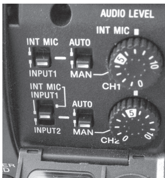
Figure 6-1 (a) The audio meters on most digital video cameras show left and right channel peak levels both currently (the bar) and in the recent past (the separated line sections giving “peak hold” functionality). This peak level is good for dialogue recording. (b) Levels for each channel are usually adjustable using audio gain controls on the side or back of the camera.
