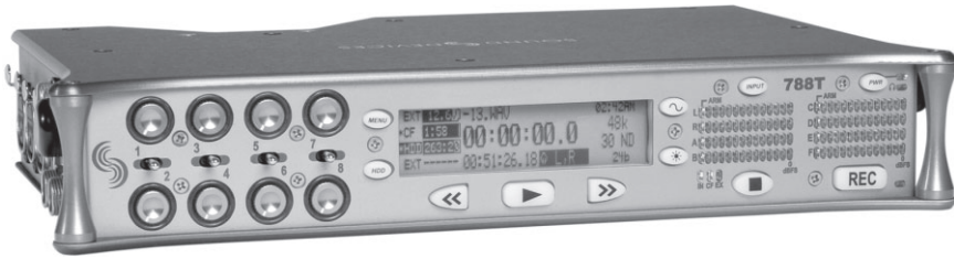
Figure 3-4 A typical high-end mixer-recorder, the 8-channel Sound Devices 788T, which adds eight-channel mixing and recording to the capabilities of similar 2-channel and 4-channel digital field recorders.
