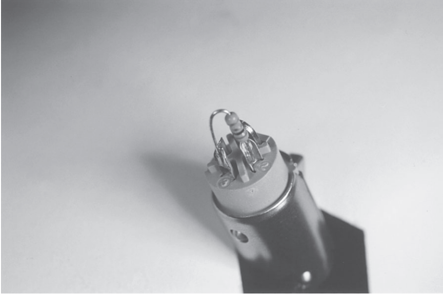
Figure 6-4 (a) In our example, a 1 k \Omega resistor is first mounted between XLR pins 2 and 3 of the male connector side of the barrel adapter.
