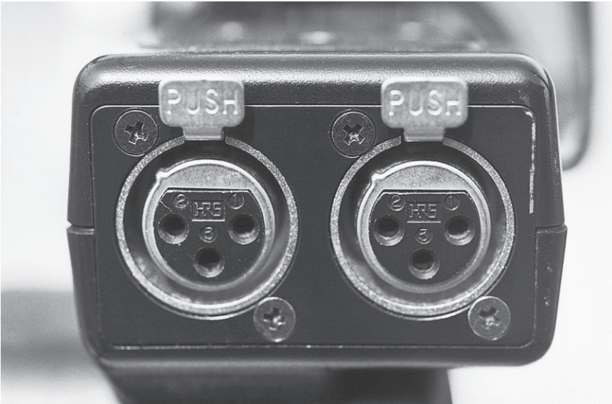
Figure 1-1 The presence of balanced input XLR connectors is the most readily apparent indication that the camera has separate microphone inputs. Note that other connector types may be used.
