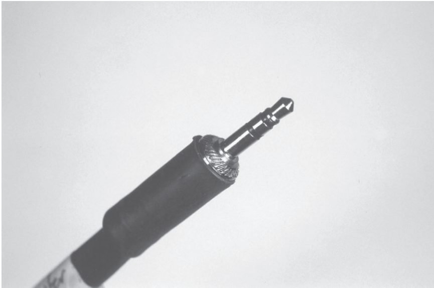
Figure 3-6 Miniature phone plug, 3.5 mm diameter, with tip, ring, and sleeve connections permitting balanced microphone or unbalanced stereo headphone connections.
