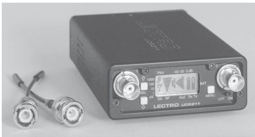
Figure 5-2 A typical radio microphone (a) transmitter and (b) receiver.
