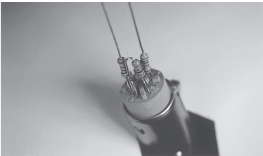
Figure 6-4 (b) Then, two 10.7 k \Omega series resistors are added as shown. The free ends are then clipped and extended with hookup wire to the corresponding pins 2 and 3 of the female connector, as is the ground, pin 1.
