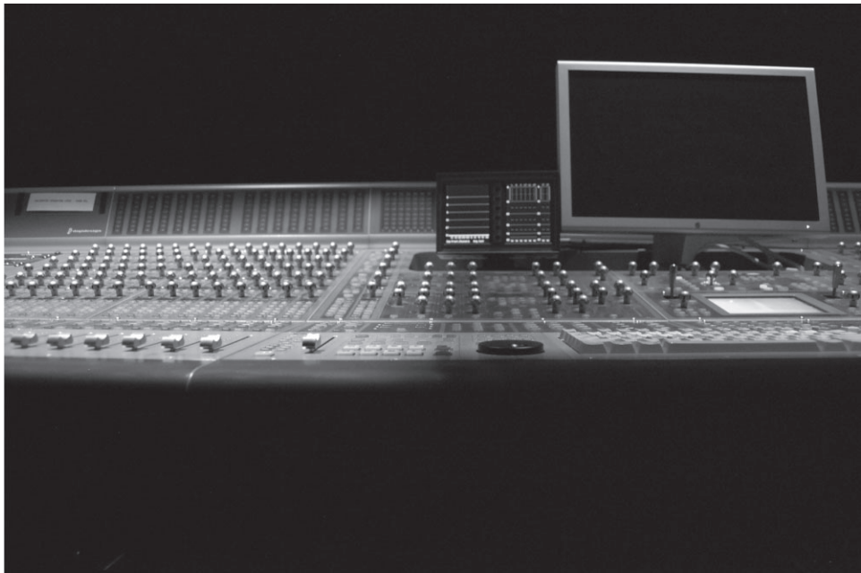
Figure 10-1 A mixing control surface with faders for controlling level and knobs for adjusting other parameters in a digital audio workstation.
