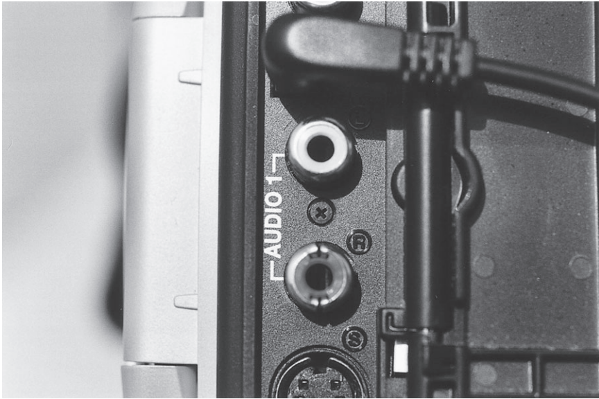
Figure 1-2 The ubiquitous consumer connector, alternatively called RCA, phono pin, or Cinch plug, and sometimes combinations of these.
