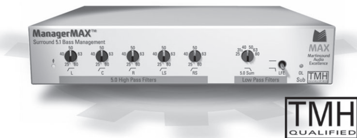
Figure 11-2 A bass manager. It high-pass filters five main channels, then sums and low-pass filters the five channels, adding the LFE signal to the sum and directing it to one or more subwoofers.
