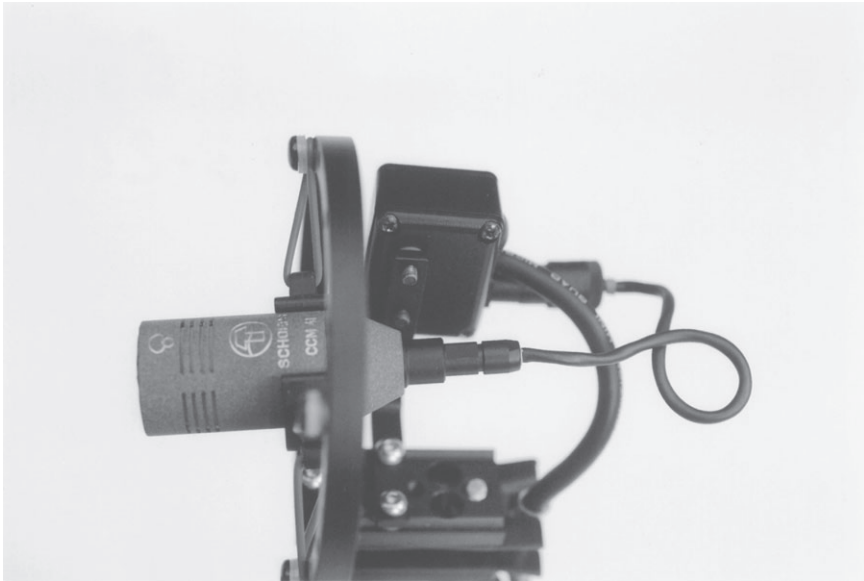
Figure 4-2b The lead dress allows the cables to be freely suspended in air—they do not touch each other nor the windscreen when the mic is in place. This particular mount uses two different cable diameters: one connected to the mic for best flexibility and one out of the assembly for ruggedness.
