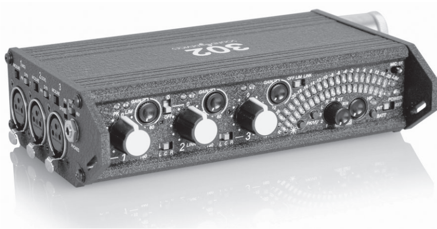
Figure 3-1 A typical over-the-shoulder field mixer for small productions, the Sound Devices 302. It has three microphone inputs and two channels of output, with dedicated level controls for each input as well as headphone level controls and other features.
