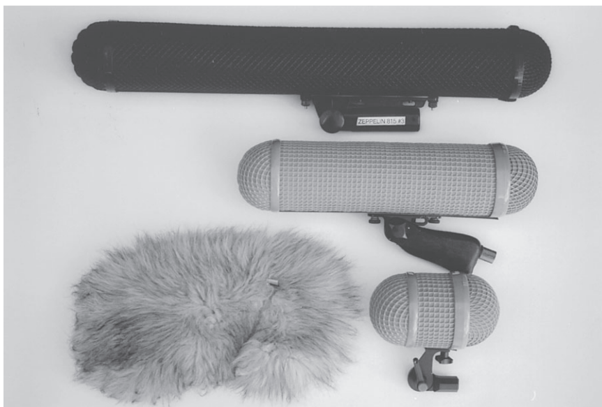
Figure 4-3a Windscreen types. Shown are differing basket-type windscreens with an internal free air volume for best performance—such types are a virtual necessity for directional mics. A Windjammer, used to cover one of the basket-type windscreens for ultimate wind protection, is shown as well.
