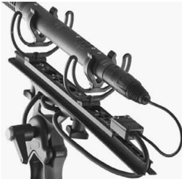
FIGURE 5.11 A lyre-shaped shock mount having different resonant frequencies in several planes.
