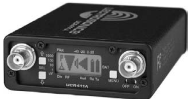
FIGURE 6.2 A radio microphone receiver for use with the transmitters shown in Fig. 6.1, a Lectrosonics UCR411A. This model includes a spectrum analyzer function described in the text. Photo courtesy of Lectrosonics, Inc.
