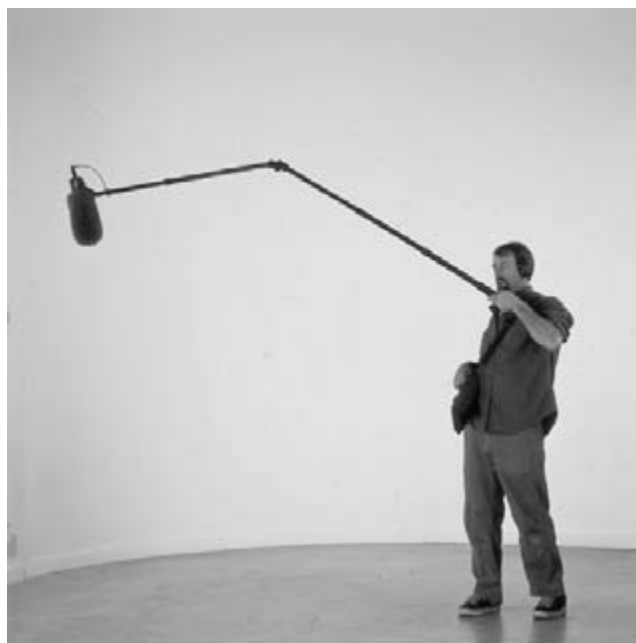
FIGURE 4.14 An articulated fishpole helps in being able to both boom and mix at the same time. Photo courtesy of K-Tek® USA, M. Klemme Technology Corp.
