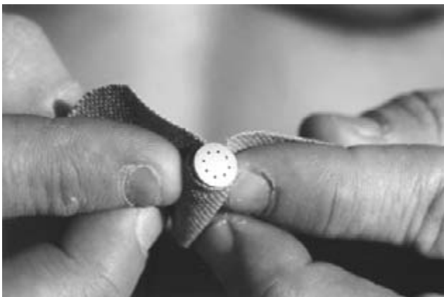
FIGURE 4.8 Wrapping a Band Aid® most of the way around a lavalier microphone will hold the lavalier in contact with the skin and not allow it to move.
