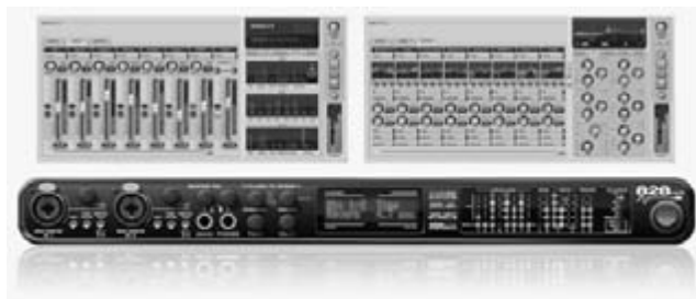
FIGURE 7.8 The MOTU 828mk3 analog-to-digital converter and FireWire interface described in the text. Photo courtesy MOTU.
