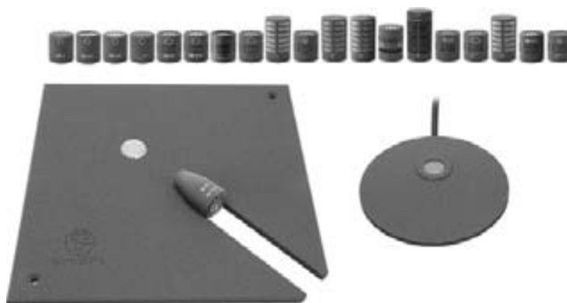
FIGURE 5.4 This series of capsules from Schoeps provides a wide variety of polar patterns and built-in frequency response variations to cover a wide range of applications. They include pure pressure (omnidirectional) and pressure-gradient (bidirectional) types, as well as cardioid, hypercardioids, subcardioids, and boundary layer types. Other variations include capsules that roll off low frequencies and ones that emphasize high frequencies, along with ones that demonstrate very flat frequency response.
